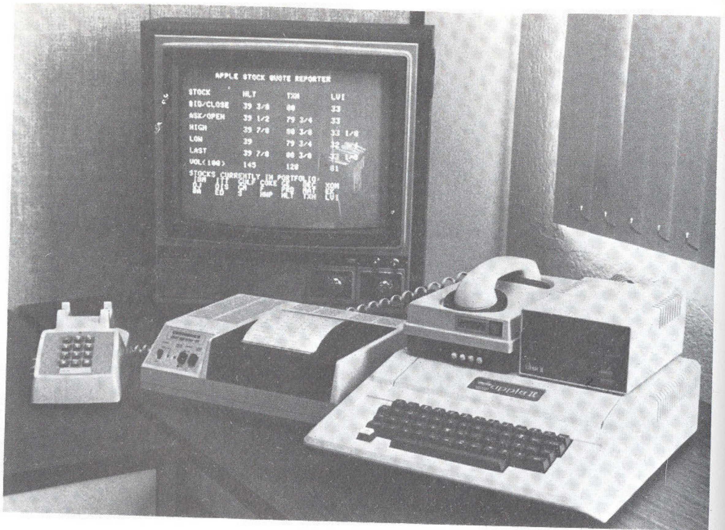
The Apple Stock Quote Reporter receives a current display of stock prices and allows the operator to place a corresponding bid. The Reporter also ascertains the closing price, the high and low price for the day, and the current volume of the stock. Stock portfolios can be easily changed to suit the individual operator.
