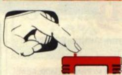
On the back of the POWER CARTRIDGE there is a Reset Button. Pressing this button makes a SPECIAL MENU appear on the screen.
