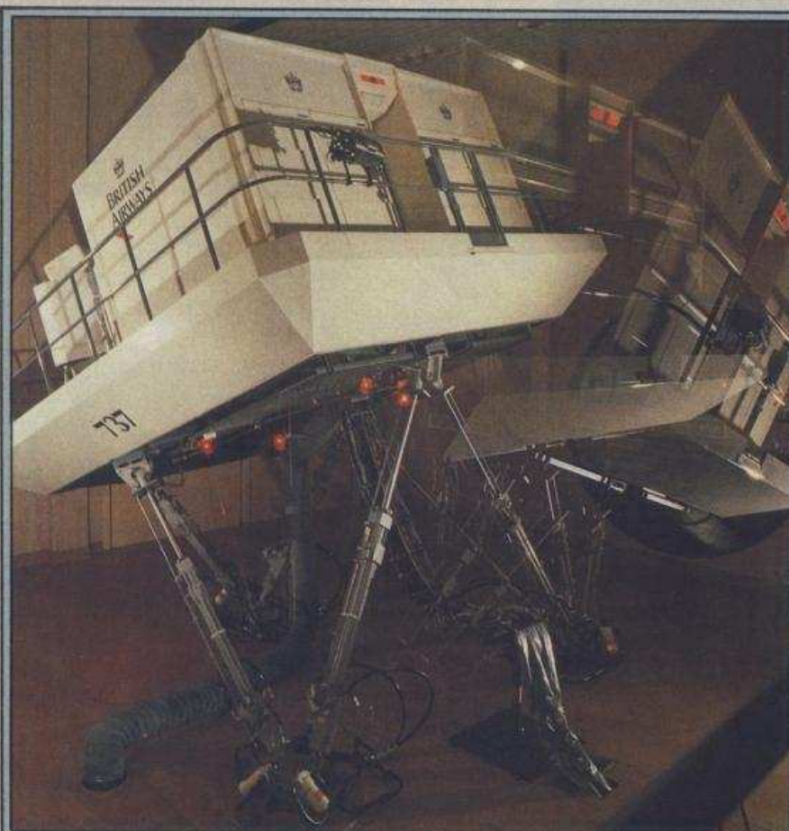
▶ Towards the future. A Boeing 737 flight simulator with Novoview SP3 visual system and WIDE display
