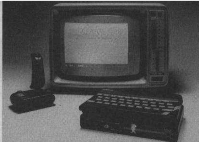
The Gamestar subscriber package includes Spectrum (48K), black box and joystick. By courtesy of British Telecom.
